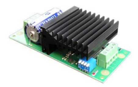
The MD03 is a medium power motor driver, designed to supply power beyond that of any of the low power single chip H-Bridges that exist. Main features are ease of use and flexibility. The motor's power is controlled by on-board Pulse Width Modulation (PWM) generators driving the H-Bridge Transistors.
